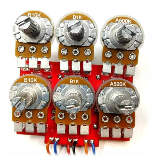
The pots connect to the PCB like this, by this stage you should have soldered the various other components - resistors, diode, transistors and capacitors etc to the board. Check your soldering over before moving forwards.
