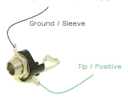
As you look at the jack in the photograph, the sleeve/ground tab is at the top, and the Tip/posi tab at the bottom.
